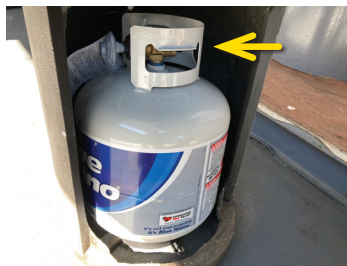
Find valve at top of tank
