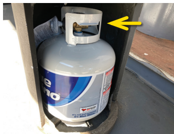
Find valve at top of tank
